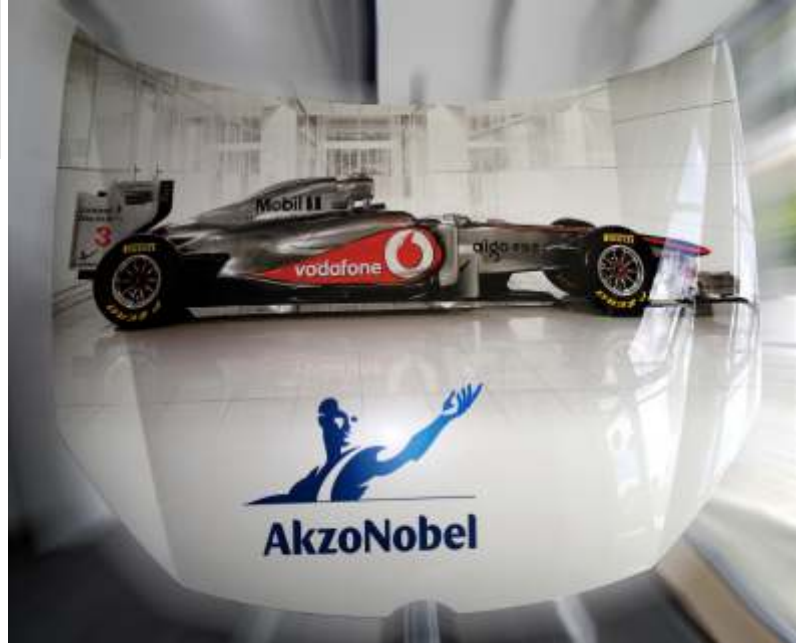
Car hood for AkzoNobel-Presentation, VAR 3D-printed, Sikkens clearcoat
